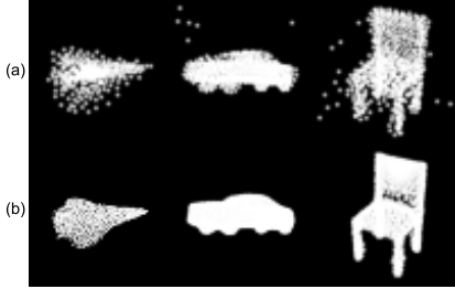
Figure 9: Projected predictions trained (a) without and (b) with affinity loss, which helps in outlier point removal.
